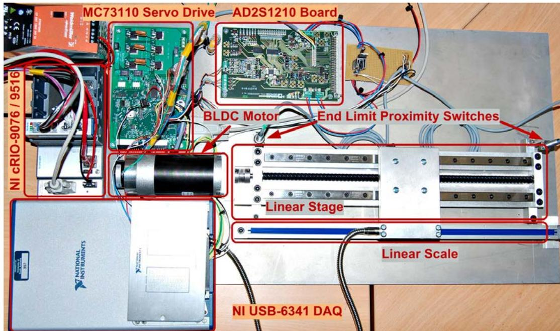
Figure 1: Hardware utilisation of the remote laboratory.
